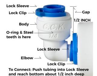
To Disconnect: Remove Lock Clip, while PRESSING Lock Sleeve Down to eliminate Gap, pull out tubing
