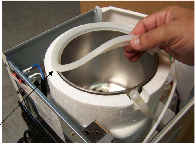
11.4 Remove the silicon over flow tube
