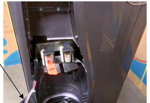
1.3 Removal of electrical connector is unnecessary.
