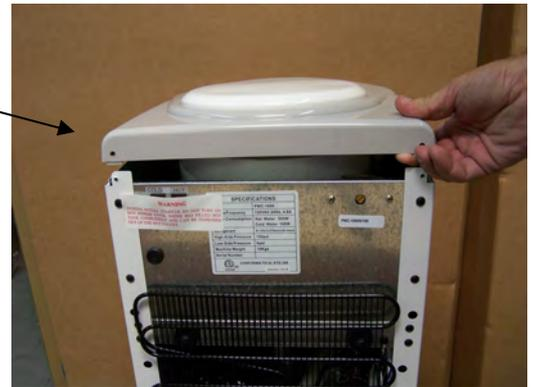
3.3 Cold tank is now accessible for cleaning and servicing other parts of the cooler.
