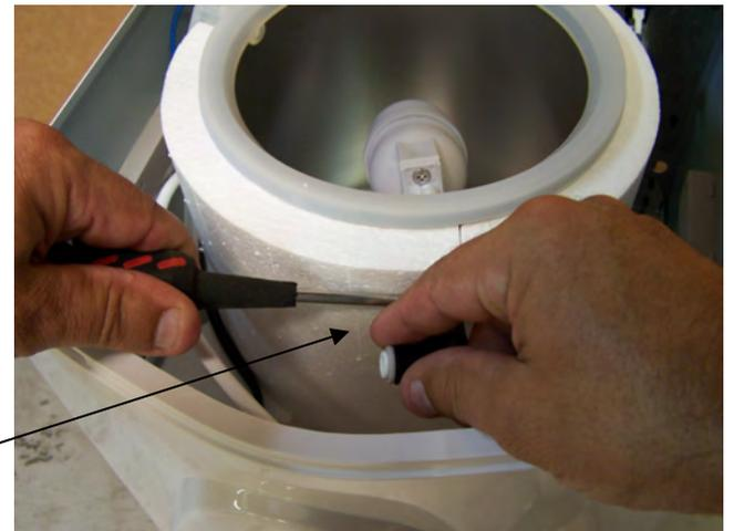
4.2 Remove elbow connector from float stem
