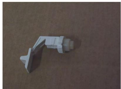
Correctly connected seal/lever assembly
