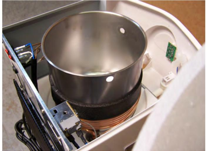
11.7 Disconnect (2) wires from sensor switch
