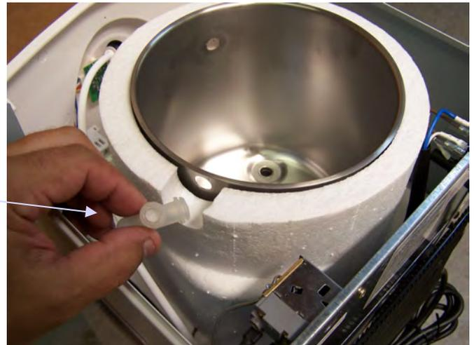
11.5 Carefully lift off the insulating foam from the cold tank
