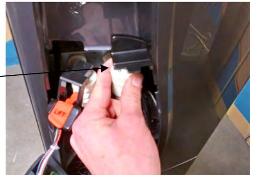
1.5 The spigot internals can now be removed/replaced.
