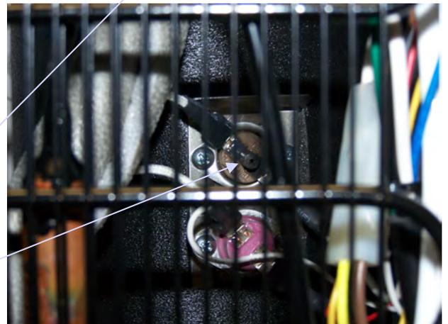
7.4 Using a long thin object such as a screw driver or a pen, depress the small black button at the center of the upper thermal switch. You should feel a click when you depress the button. This action resets the over-temp sensor.
