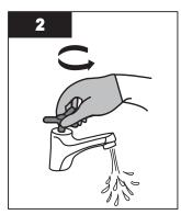
Open a tap downstream of the UV unit to release pressure. Then, close this tap.
