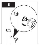
• Remove the UV sensor by grasping the body of the sensor and rotating it counter-clockwise.
