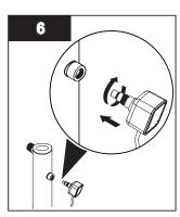
• Install the new UV sensor until a water-tight seal is achieved.
