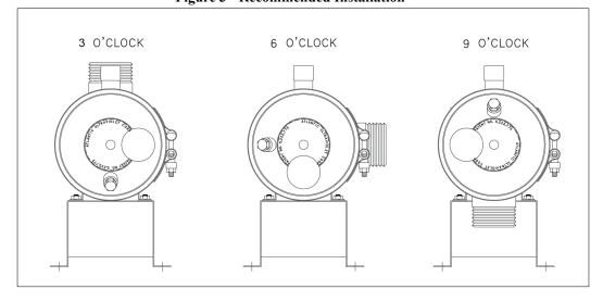
Figure 3 - Recommended Installation
