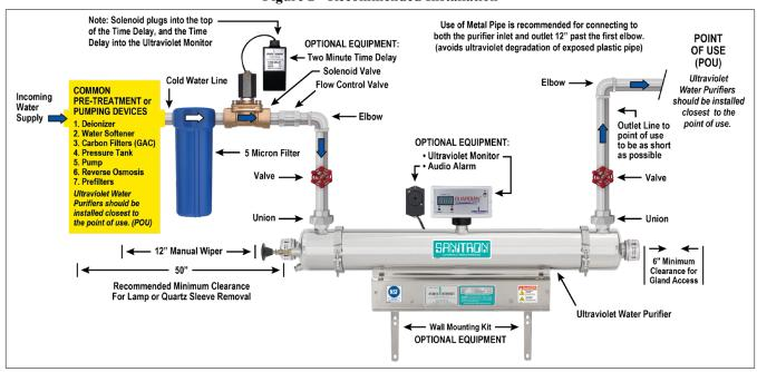
Figure 2 - Recommended Installation
